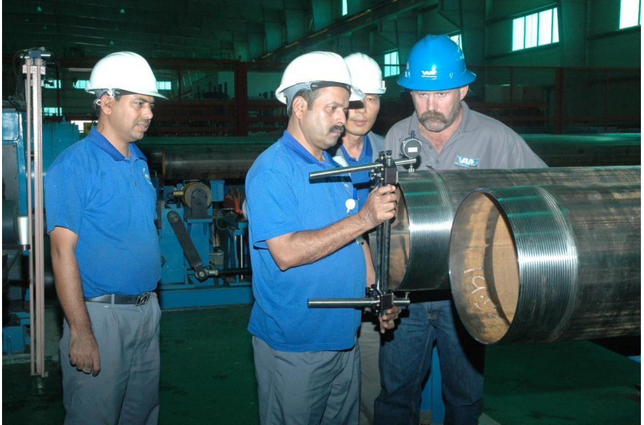
EXPERT HANDS: K55's are high-tensile casing pipes equivalent to X80 steel grade that is conventionally used in deep well applications and until now are being imported from foreign pipe producers.
